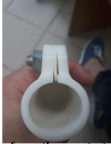
Fig. 10. Delamination of the handle
